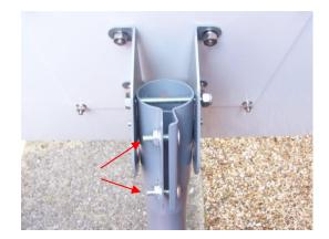
Figure 4-16 - Adjusting azimuth
