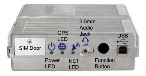
Figure 1-6 – Front side view of IDU
