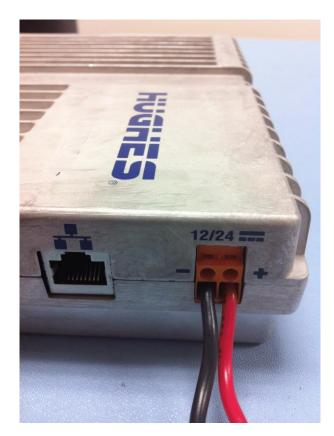
Figure 4-9 - Connecting power leads
